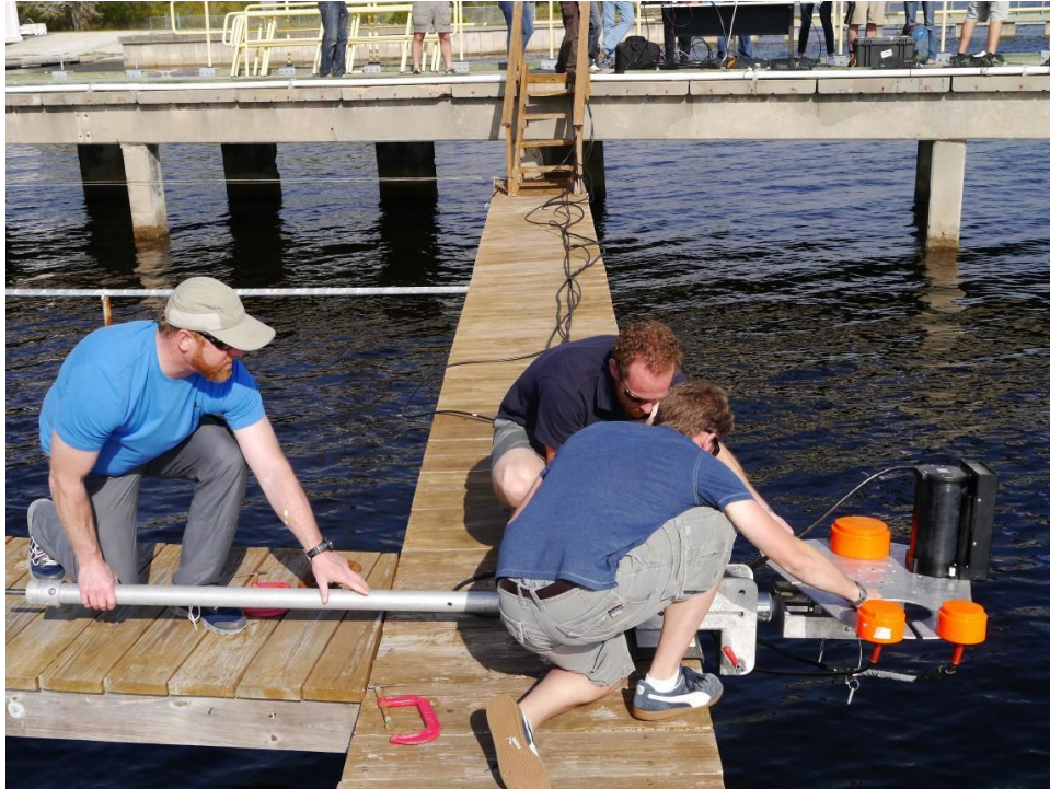
Meeting attendants deploy four, pole-mounted sonar transducers into the shallow waters of St. Andrew Bay: Two SIMRAD EK60s (200 and 333 kHz), a SIMRAD EK80 (100-150 kHz) and a Sound Metrics DIDSON model 300 m.
