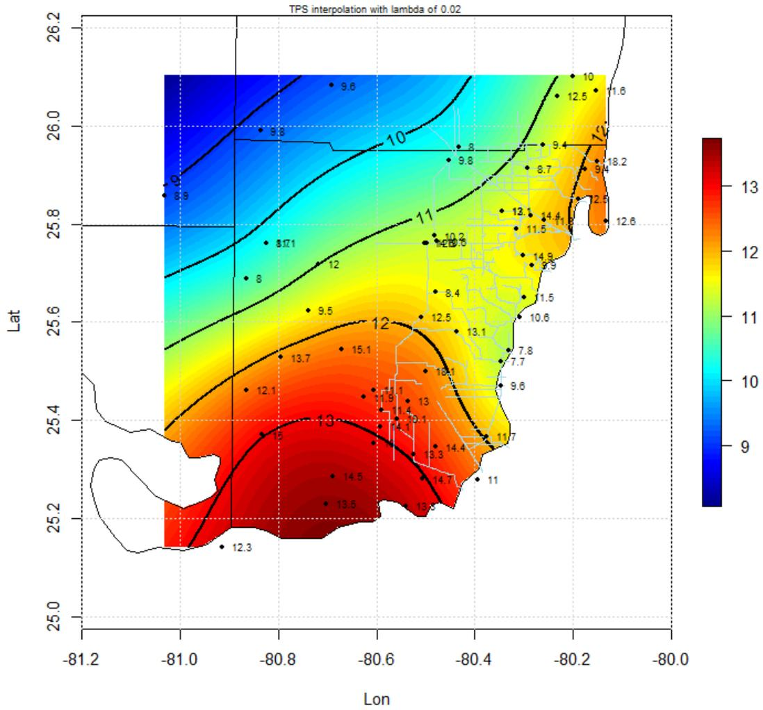
Figure 8. 1-in-100-year 3-day rainfall totals (inches) based on thin-plate-spline (TPS) smoothing of station data (in black).
