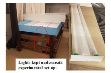
6) By now, the holding chamber and observational chamber should be filled with aerated, heated water, the camera set and the source of light turned on. Next, enclose the experimental set-up with the blackout curtain and secure using a clip.
